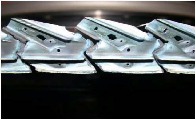
HP turbine blade showing gross erosion of shroud and front seal fin
