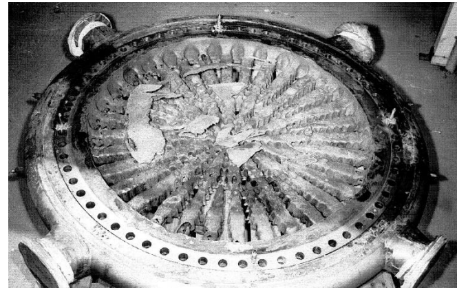
Injector face destroyed by combustion instability, Source: D. Talley
