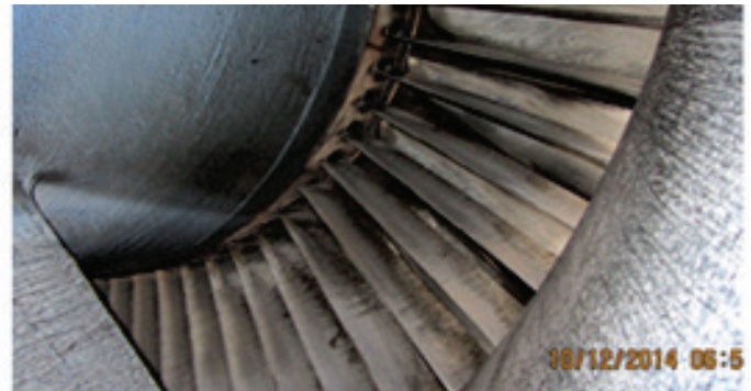
Figure 10: F8 Filtration after 5,000 Hours (Two Offline Washes)
